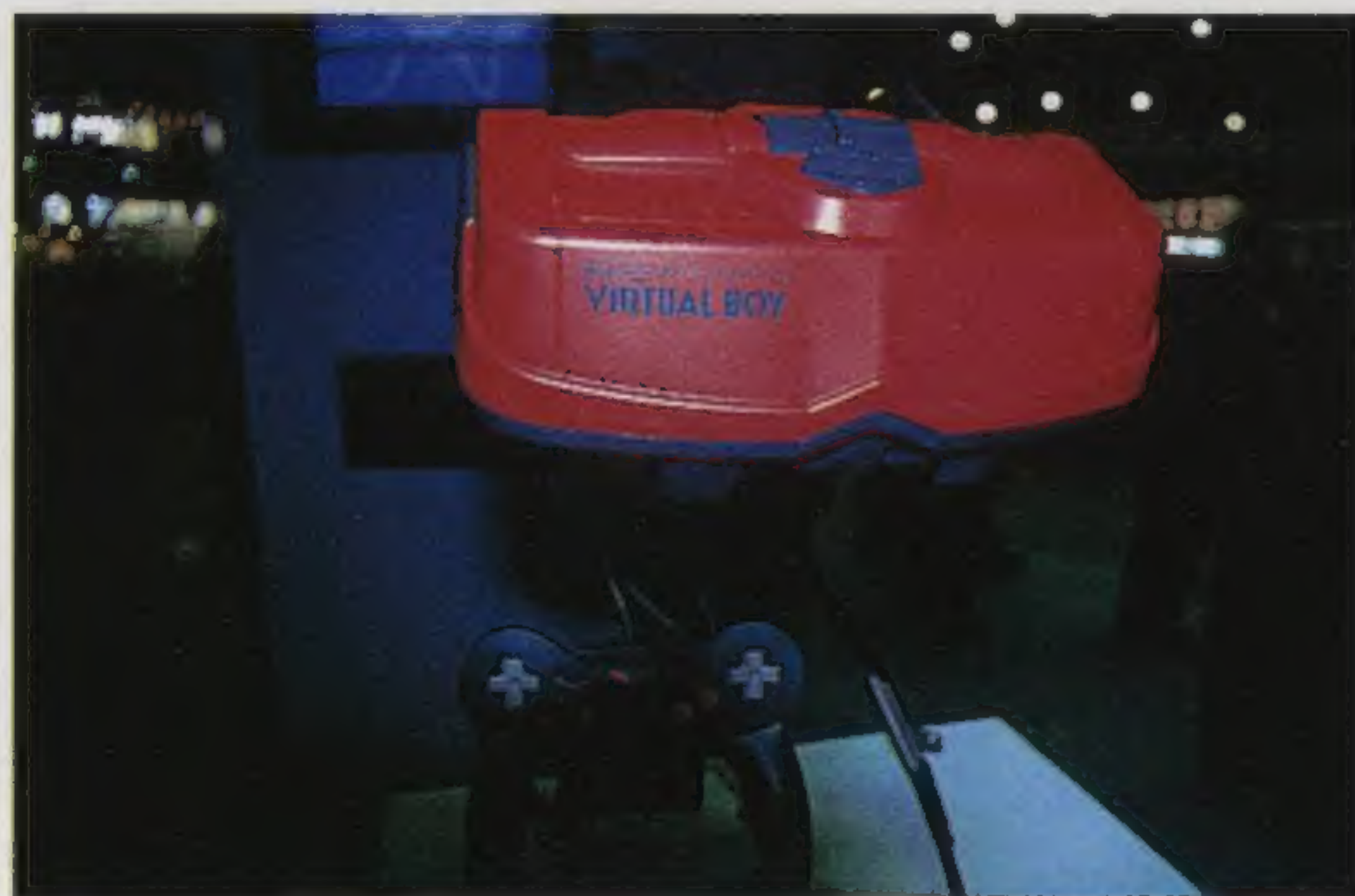
The Virtual Boy hardware has a red and blue body. A joystick with elongated handles is attached via a lead
